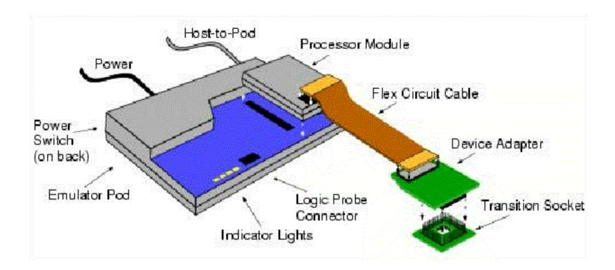
The emulator pod connects to the PC through either a parallel port or a USB port. The pod contains the hardware necessary to perform the common emulator functions, such as trace, break and emulate. It also permits the communications between PC and processor module
