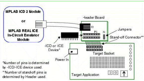
A special ICD or ICE device is connected to a header board to be used with the ICD 2 in-circuit debugger or REAL ICE in-circuit emulator. This device is mounted on the top of a header and its signals are routed to the debugger or emulator connector. On the bottom of the header is a socket that is used to connect to the target board
